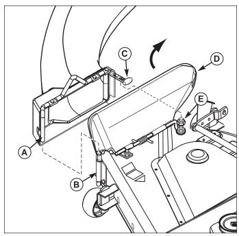
Figure 12. Install Lower Tube
